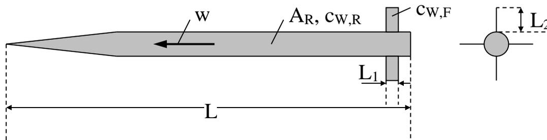
geg:  $w = 600 \text{ km/h}$        $A_R = 1,48 \text{ m}^2$        $L = 2,7 \text{ m}$
