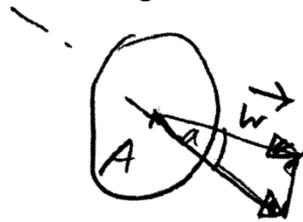
$$\begin{aligned} \dot{m} &\sim A \\ \dot{m} &\sim \rho \\ \dot{m} &\sim w \cdot \cos \alpha \cdot \rho \cdot A \end{aligned}$$
